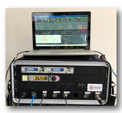
The system comes fully mounted and calibrated in a transportable Gator 3U or 4U (depending on the options on number of receivers) Light Weight Rack Bag.
